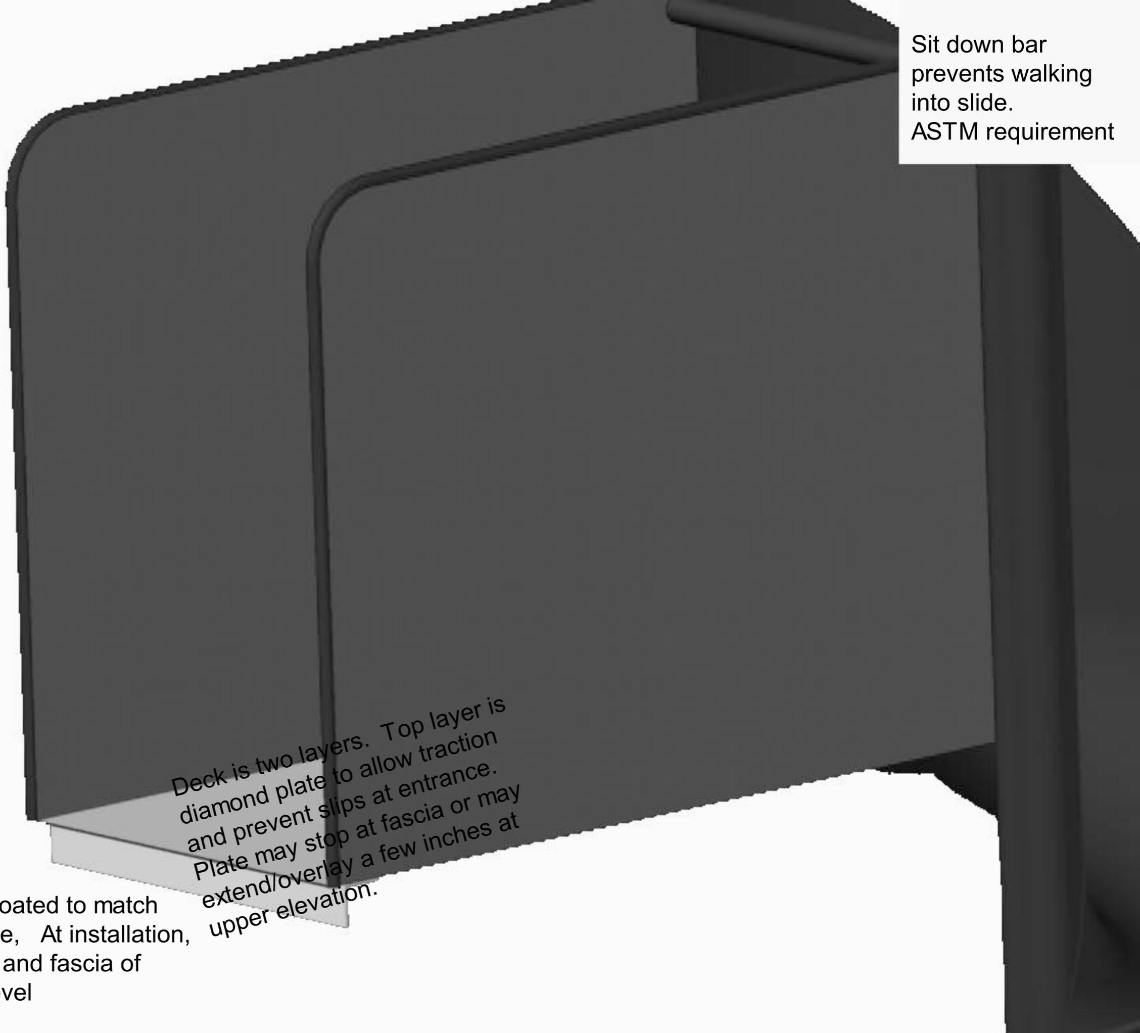
Many of our designs request the ability to configure the entrance/transition deck to be able to easily attach to the barriers present on the upper elevation. This design modification/option allows for each attachment to a squared edge such as a terminus post on the barrier. Create an opening at your upper level, insert O.D. of the box into the I.D. of your opening and bolt to attach or close
